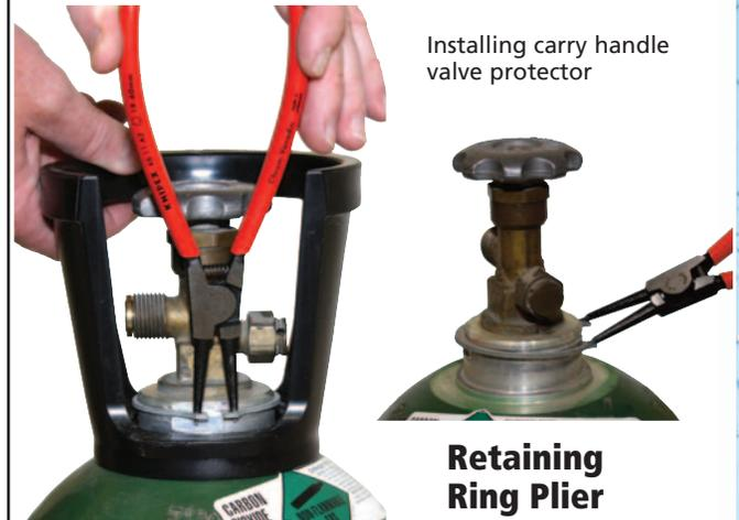
Installing carry handle valve protector
